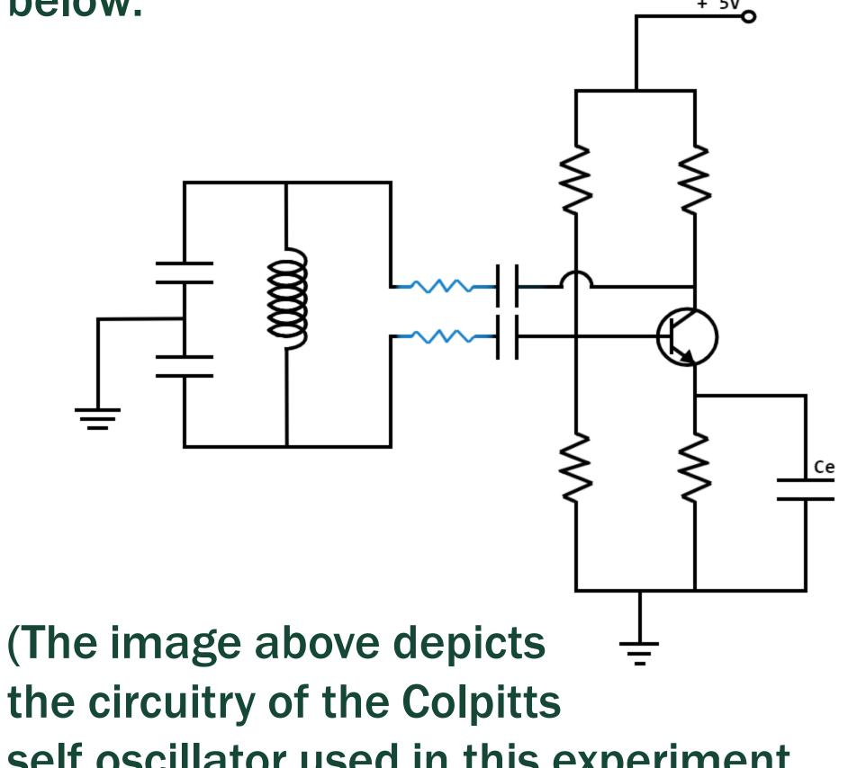
self oscillator used in this experiment, with the tested resistors highlighted in blue.
