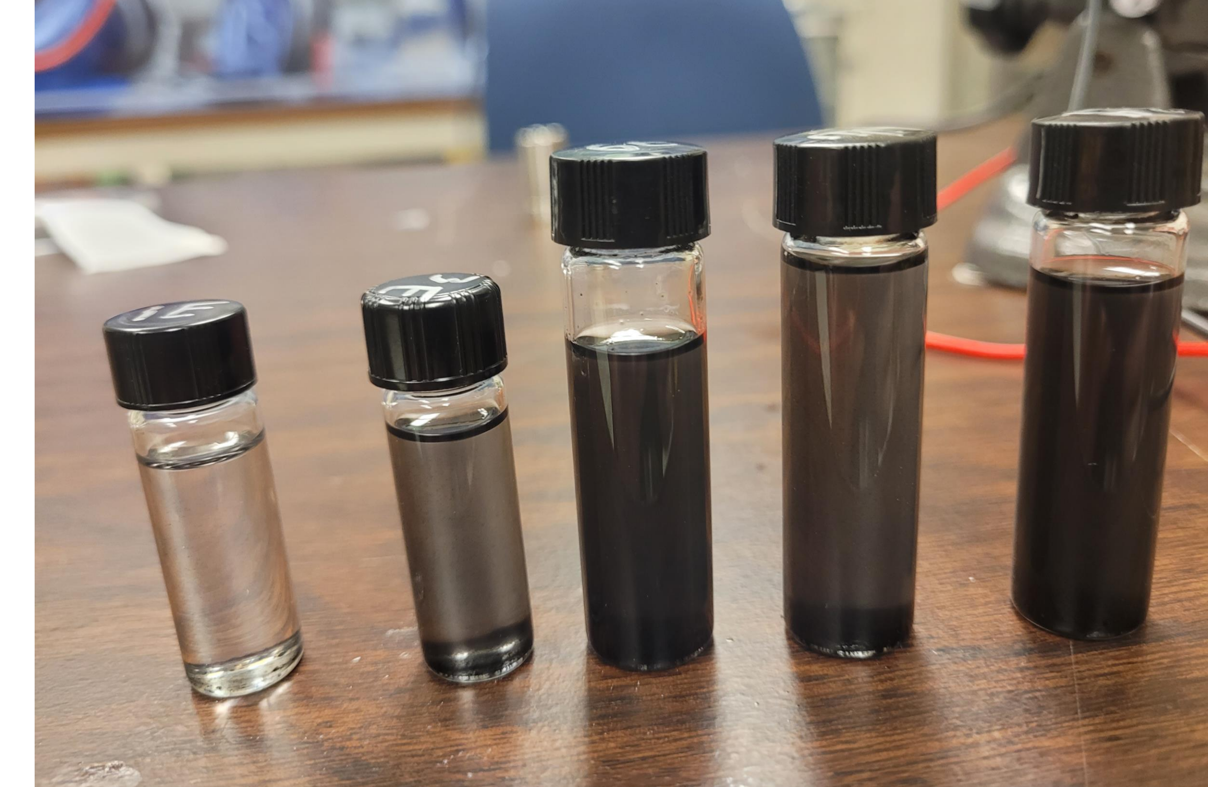
Figure 2: Samples of Powdered Activated Carbon in Liquid Scintillation Cocktails
