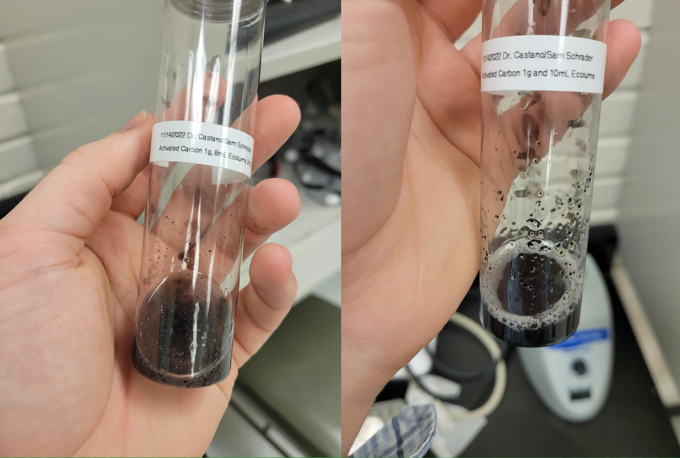
Figure 1: Samples of Activated Carbon in Liquid Scintillation Cocktails
