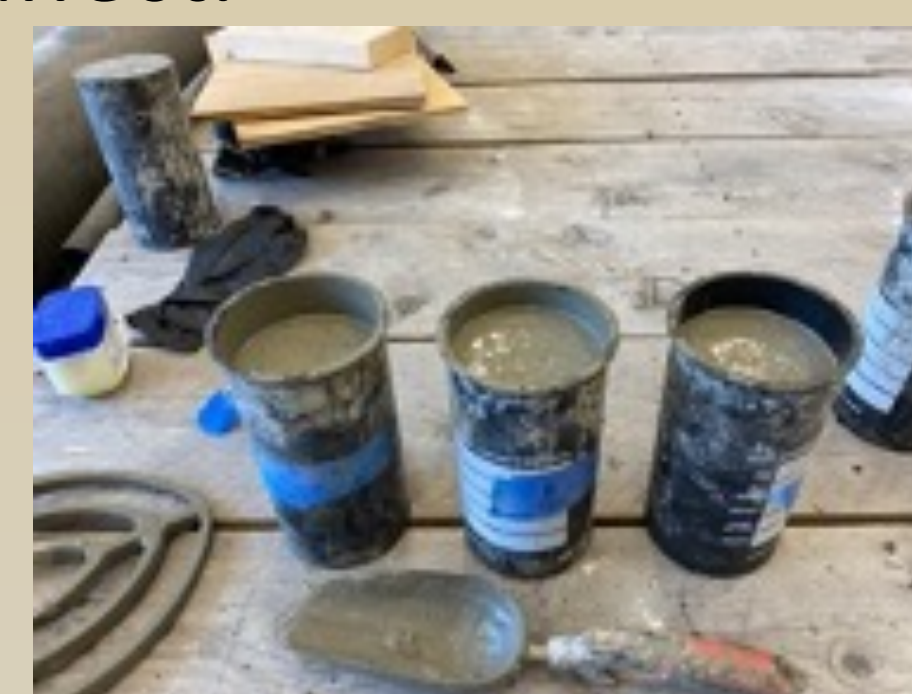
Fresh poured UHPC cylinders
