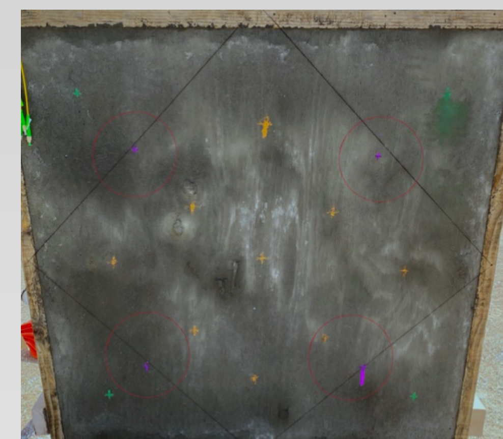
Ballistic Testing on Concrete Samples
