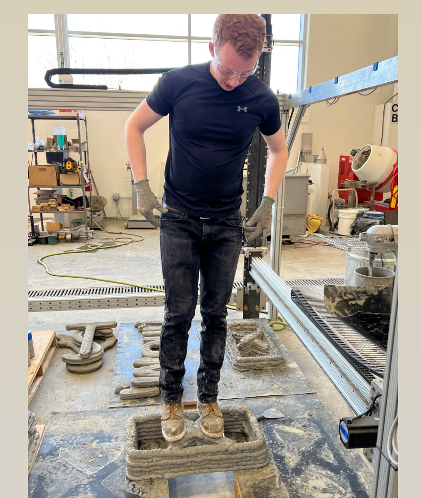
Printed UHPC wall structure
