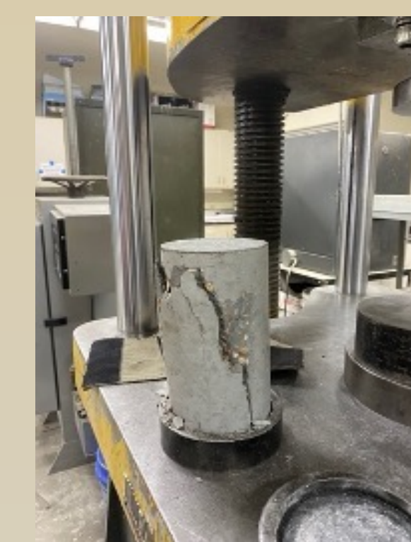
UHPC Cylinder After Compression Testing. Compressive testing hit over 8000 psi
