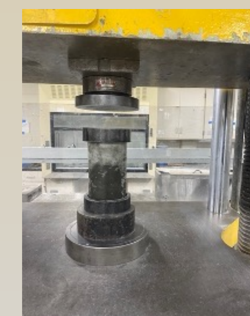
Poured compression test cylinder
