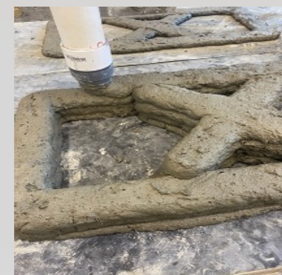
Printable UHPC Wall Structure
