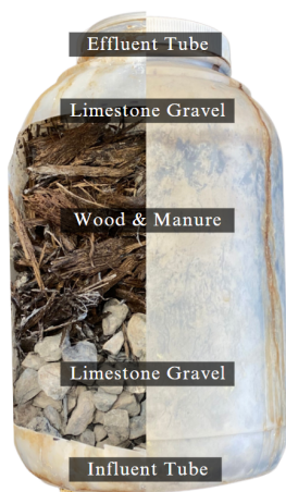
Figure 1 : Bioreactor Cross-Section
