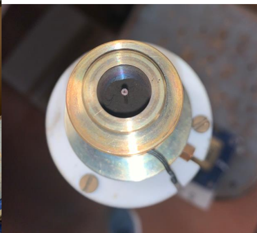
Figure 4: View from the top into the toroid-cavity pressure vessel filled with powdered catalyst
