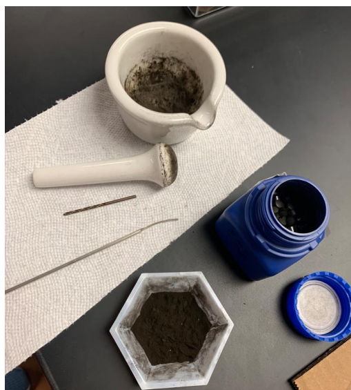
Figure 2: Procedure to obtain the Cu-ZnO/Al 2 O 3 catalyst in powdered form.
